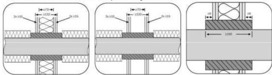
For timber stud partitions, seal must be ≥100mm from studs with ≥100mm of insulation (A1 or A2 to EN13501-1) between seal & stud. For further details check the ETA.
