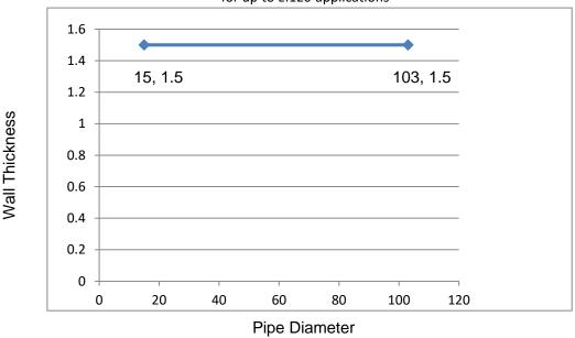
D.2 Field of application for minimum 250mm long Tenmat Firefly 109+ LP Fire Sleeve – Circular (Standard Sleeve) for PVC-U circular ambient pressure extraction and ventilation 'duct' type pipes penetrating minimum 100mm thick fire resistant walls for applications up to El120:
