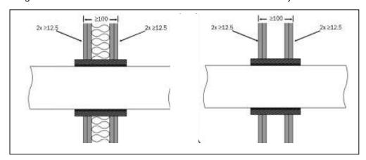
The seal must be a minimum of 150mm long with 25mm protruding each side
