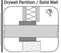
Rigid walls must comprise concrete, aerated concrete or masonry ≥650kg/m³ (Wall Type A) or concrete , masonry ≥1100kg/m³ (Wall Type B)
