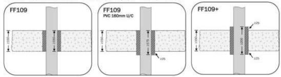
Rigid floors must comprise concrete ≥2400kg/m³ (Floor Type A) or ≥550kg/m³ (Floor Type B). For further details check the ETA
