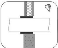
Rigid walls must comprise concrete, aerated concrete or masonry ≥650kg/m³ (Wall Type A) or concrete, masonry ≥1100kg/m³ (Wall Type B)
