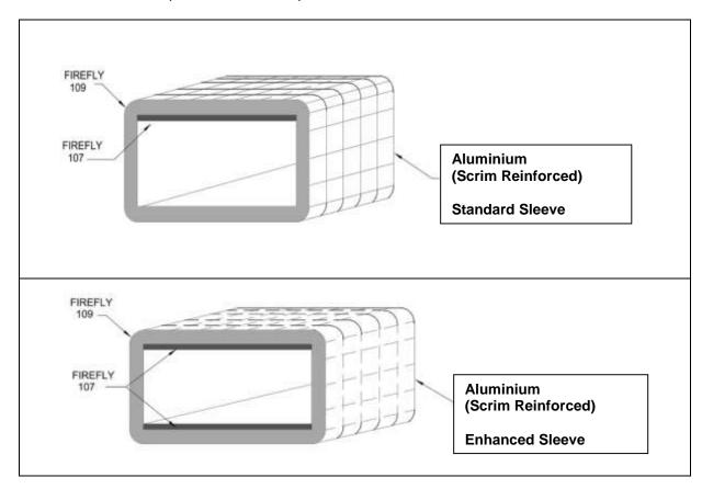
The Firefly 109+ LP Fire Sleeve – Rectangular is delivered in various sizes to fit particular duct sizes – see table below:
