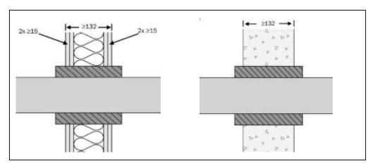
The seal must be a minimum of 180mm long with 24mm protruding each side of the wall
