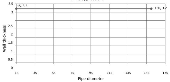
C.1.3 The line graphs below show the coverage of the allowable HDPE (according to EN 1519-1)\* pipe diameters and wall thickness for applications up to El120: (any pipe size variation along the line is covered)
