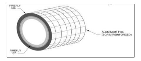
The Firefly 109, 109+ and 109+ LP Fire Sleeve – Circular is available as single sleeve up to 500mm long which can be cut down to suit the intended application. It must be a minimum of 150mm long or longer if the wall is thicker. The Firefly 109, 109+ and 109+LP is delivered in various sizes to fit particular pipe diameters – see table below:
