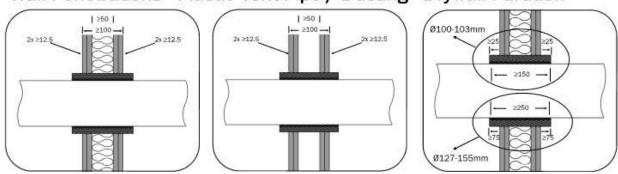
For timber stud partitions, seal must be ≥100mm from studs with ≥100mm of insulation (A1 or A2 to EN13501-1) between seal & stud. For further details check the ETA
