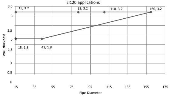
B.2.2 The line graphs below show the coverage of the allowable HDPE (according to EN 1519-1)\* pipe diameters and wall thickness for applications up to EI120: (any pipe size variation along the lines and the area between the lines is covered)
