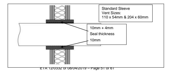
D.6 Field of application for Tenmat Firefly 109+ LP Fire Sleeve – Rectangular (Enhanced Sleeve) for use with a 220mm wide x 90mm high PVC-U rectangular ambient pressure extraction and ventilation 'duct' type pipe penetrating fire resistant walls for applications up to El120:
