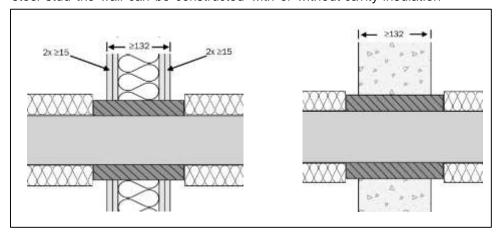
The seal must be a minimum of 150mm long with 9mm protruding each side of the wall
