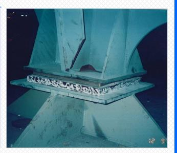
**TENMAT** has successfully supplied over 70 tankers (to date) with *FEROFORM* F3637 tanker pad system without a failure. In more than 25 years in service FEROFORM has always outlasted the ship's life, thus TENMAT has never supplied a spare part; FEROFORM F3637 pads are maintenance free.
